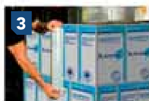
3 Hold the film parallel with the corner of the pallet before you lock it off with the palm of your hands or thumbs.
