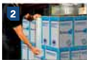
2 Let the film unwind freely until you reach the point (before the container) where you need to apply tension
